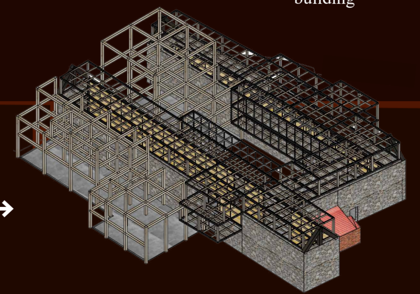
4. Secondary steel frame building
