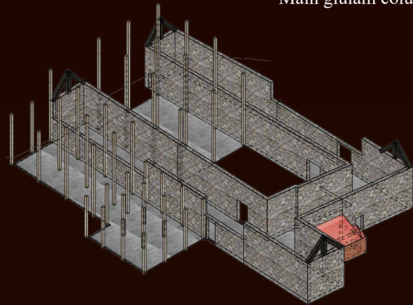
2. Foundation building & Main glulam columns
