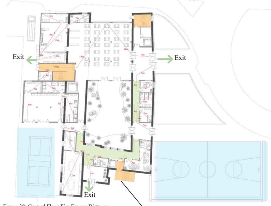
Figure 38: Ground Floor Fire Escape Distance
